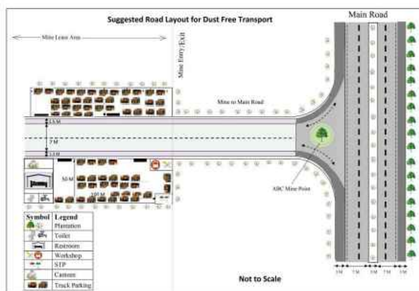
Fig. 12.1: Schematic Diagram of Suggested Parking Plazas Inside the Mining Lease Area with Connectivity to Main Road from Mine to Main Road
