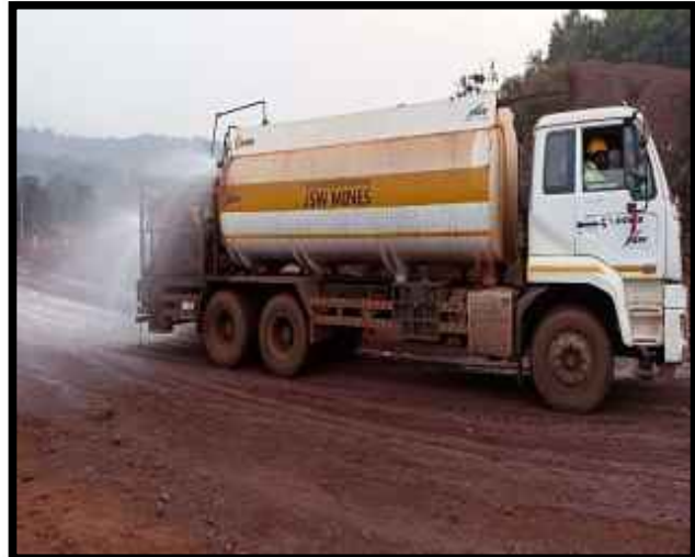
16KL WATER SPRINKLER
