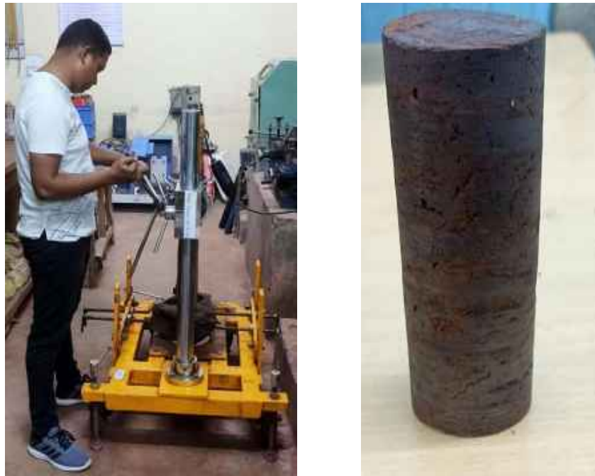
Figure IV. Coring operation and cored specimen
