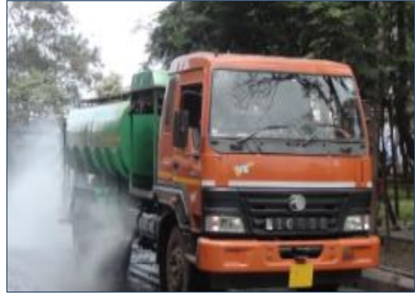
Truck mounted water tanker for water sprinkling
