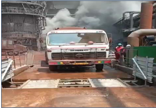
Wheel Washing facility
