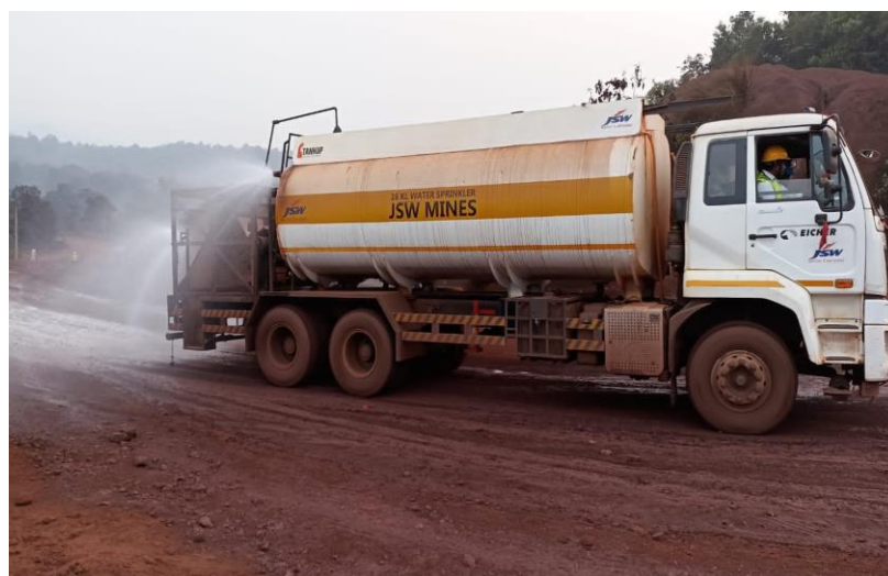
Water Tanker Arrangement for Haul Road Dust Suppression
