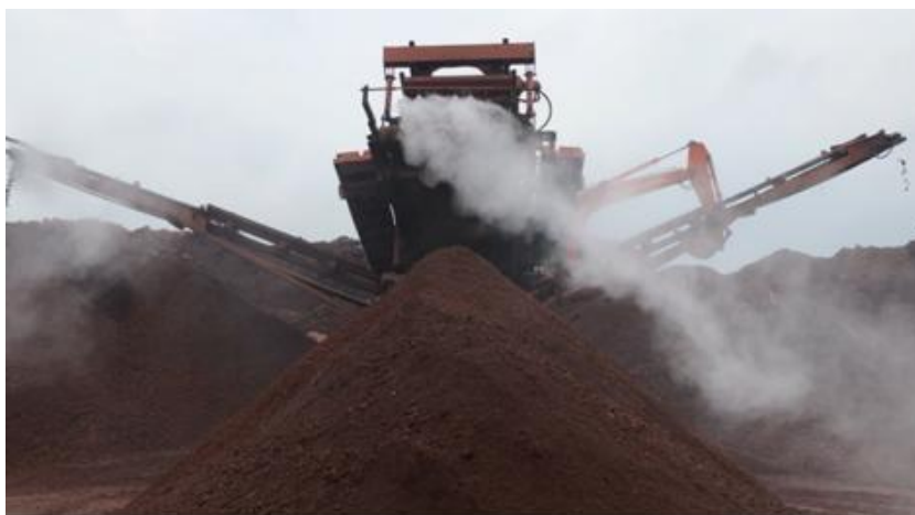
Dry Fog System in Mineral Handling Plants
