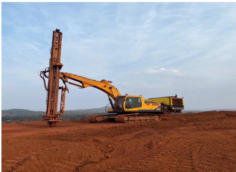
Wet Drilling and Dust Extractor System in Drilling Operation
