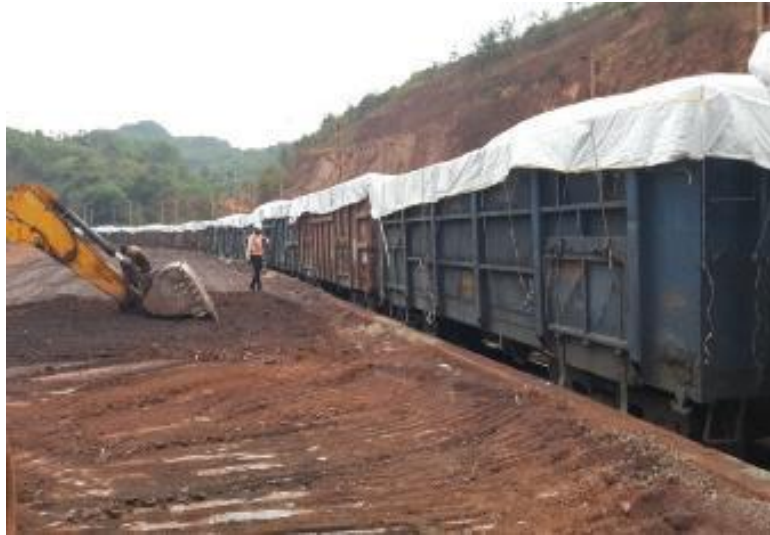
Tarpaulin Covering on the Railway Wagons
